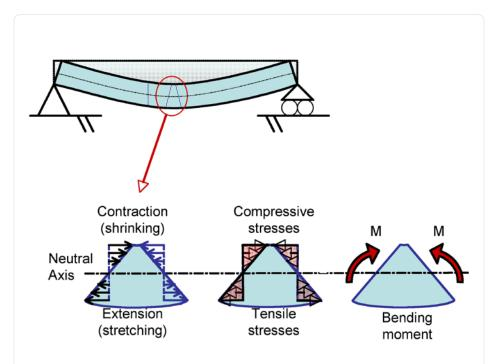
**Fig. 1.** A schematic relating curvature to bending stresses and eventual bending moment.
