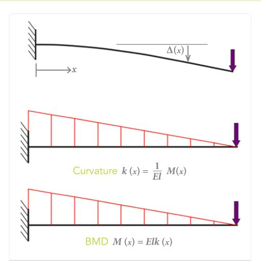
**Fig. 1.** A deflected cantilever along with the corresponding bending moment and curvature diagrams accompanied by the associated equations.
