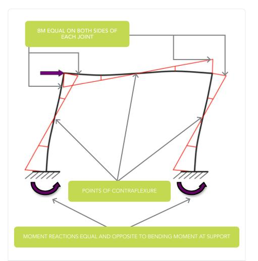
**Fig. 2.** A fixed portal frame deflecting under a horizontal load applied to the top left corner. The bending moment along the beam has then be sketched in red with annotations to explain trends.
