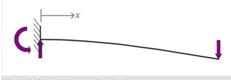
Fig. 1. Deformed shape and load and reactions.
