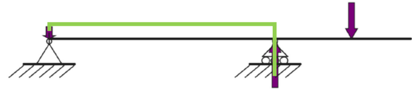
Fig 7. The shear force changes direction on meeting a force in the opposite direction.
