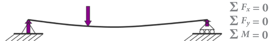
Fig. 1. The 2D equilibrium equations necessary to find the reactions of an (isostatic) simply supported beam.
