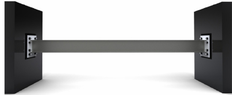
Fig 12. Encastré Beam Push Me Pull Me model
