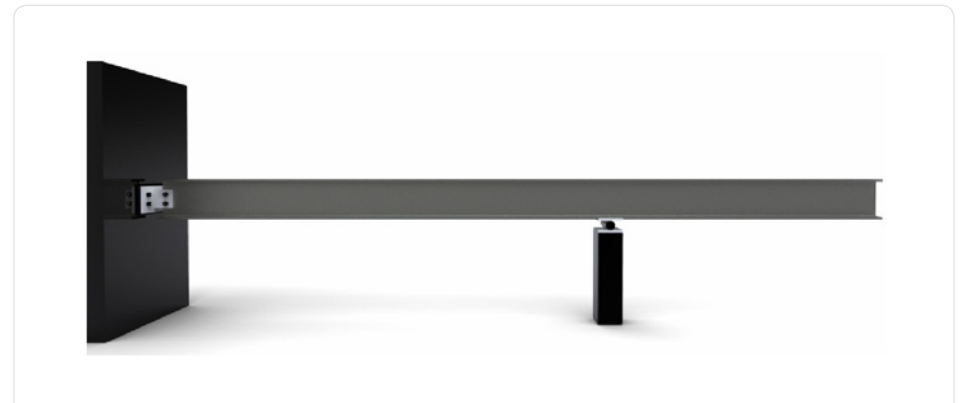
Fig 8. Simply Supported Beam with Cantilever Beam End Push Me Pull Me model.
